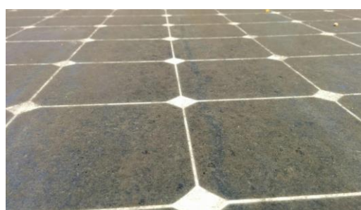
Figure 28. Dust on Mono-Si panel
