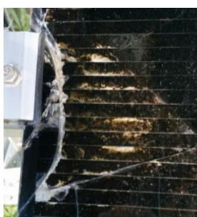
Figure 29. Broken CdTe solar panel
