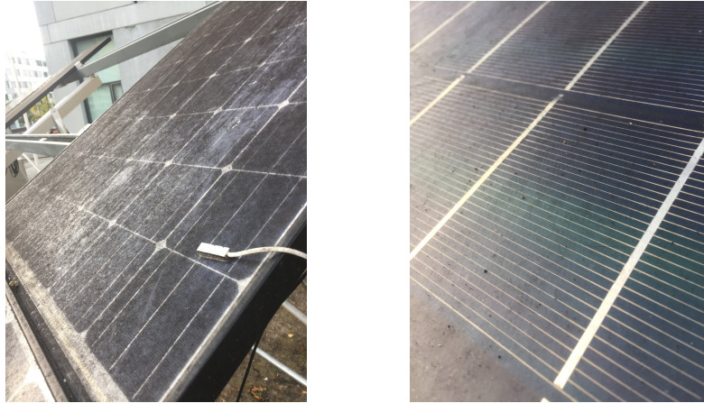
Figure 4: Thin but heavily caked on dirt from ten months can be seen on the CIGS with back mirror, Module 6, while Module 1 the flexible CIGS panel shows small, sparse, sappy dots (pictures taken 13th October 2016).
