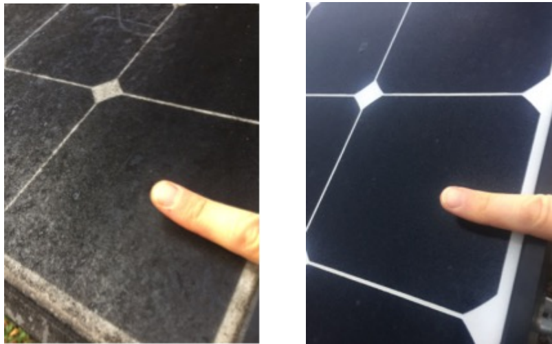
Figure 6: Before and after cleaning the back contact monocrystalline silicon module.
