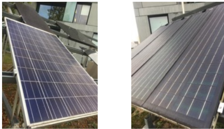
Figure 2: (a) Glass-covered polycrystalline silicon and (b) flexible-bodied epoxy CIGS at AMOLF, Netherlands.
