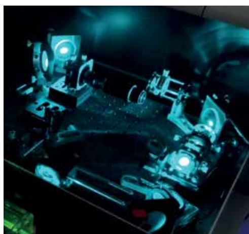
Today's multi-color single-molecule TIRF microscope K2 (Simultaneous Triple-color total Internal Reflection Fluorescence).
