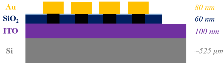
Figure 4.1: Final device architecture. All of the materials are listed in the correct order and their thicknesses are provided. Self-assembled monolayer of OTS is depicted as a very thin blue line on top of the SiO 2 layer.
