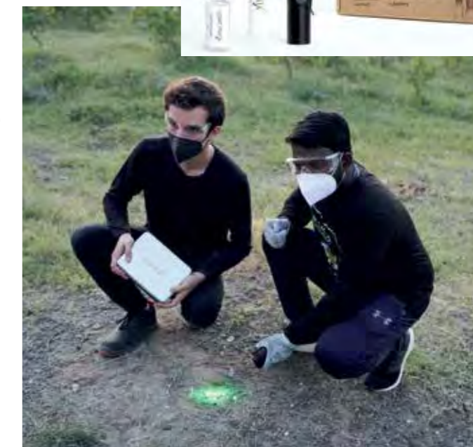
Use of the Lumetallix test kit in the field.
