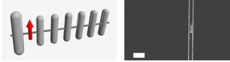
Fig. 3.14 Left: cartoon of a Yagi-UDA antenna. For radio and TV waves such an antenna is meter sized, and consists of a single active element (red arrow, connected to current receiver/source) and a set of rods mounted on a linear mechanical support (thin rod). The vertical rods are cut to approximately \lambda/4 length, and the antenna pitch is at most \lambda/3 . The longer rod is called ‘reflector’, while the set of smaller rods are called ‘directors’. When driven (current through red element, which alone would be an isotropic radiator), the antenna radiates strongly along the axis of the antenna while no radiation emerges on the reflector side. Right: scanning electron micrograph of a Yagi-Uda antenna with a response at optical wavelengths. The total length of the structure is just 1 micron. The five gold particles (reflector on lower side of antenna) are fabricated using electron beam lithography on top of an optical waveguide, which is a 500 nm wide silicon nitride strip on a quartz surface. The antenna can interface nanoscale sources and detectors to guided modes that propagate in the dielectric strip.
