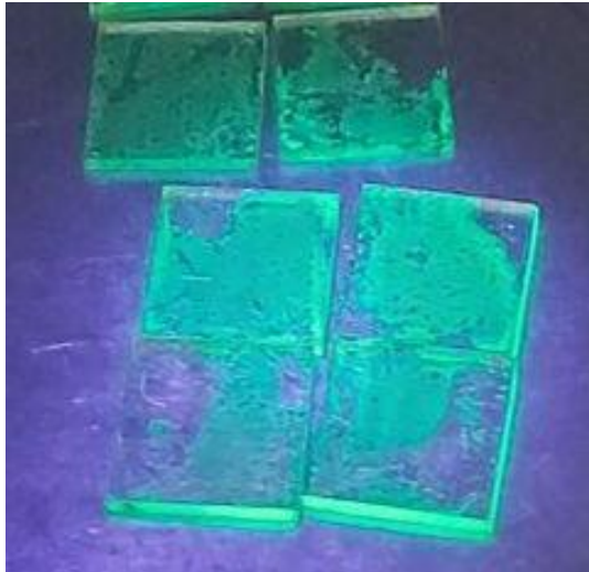
Figure A.2: A picture of patterned substrates after perovskite deposition. Substrates are observed under UV light to induce the photoluminescent emission observed.
