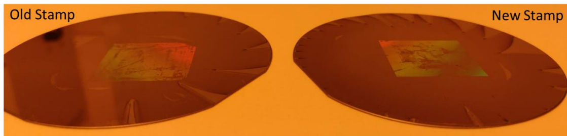
Figure 4.8: A picture of 2 silica wafers stamped using the “old” (left) and “new” (right) stamp. The observed squares highlight the patterned areas.
