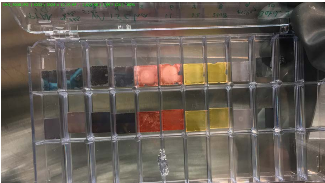
FIGURE A.4: Perovskite layers MaPbI_3 , MaPbBr_3 and mixed MaPbI_xBr_{1-x} in different ratio's ( x = 0.2, 0.4, 0.6, 0.8 ). On the left: pure MaPbI_3 , on the right: pure MaPbBr_3 .
