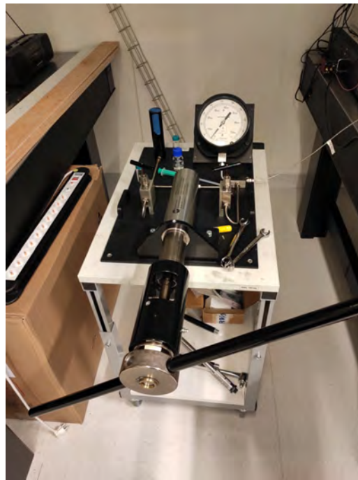
Figure B.1: The pressure cell in figure (a) and the manual pump to generate pressure in figure (b)
