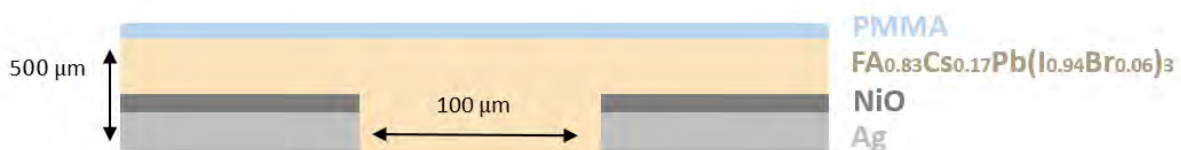
Figure 4.2: Sketch of device lateral section. The sketch is not in scale. The Si layer is expected to be 100 nm thick, the NiO layer is roughly 10 nm thick.
