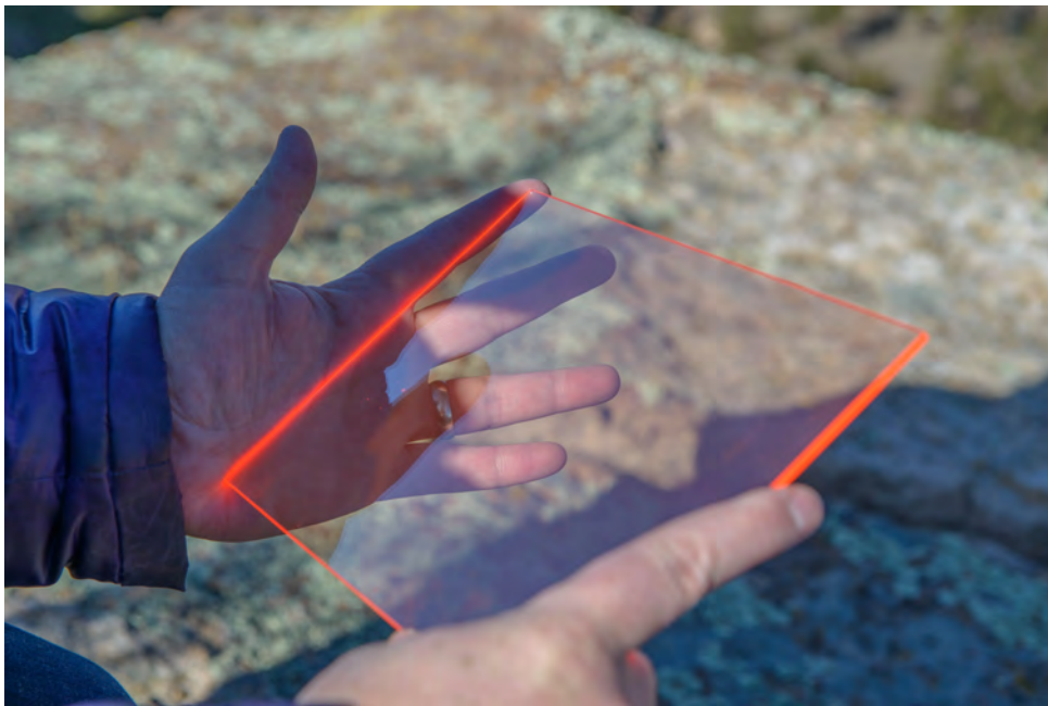
FIGURE 1.2: Photo of an LSC built by UbiQD. The LSC is mostly transparent, with a concentration of the absorbed light directed to the edges, causing them to glow red. Image retrieved, with permission, from UbiQD's Twitter page [6].
