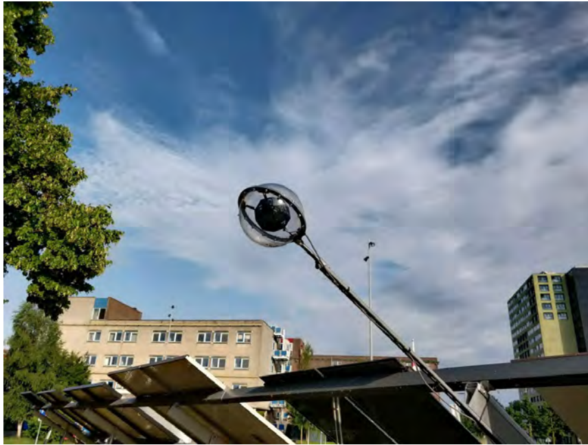
FIGURE 3.4: The 12-sided LAD situated in the solar field at AMOLF. It is encased in a clear, spherical protective plastic shell that is heated to prevent a build-up of condensation.
