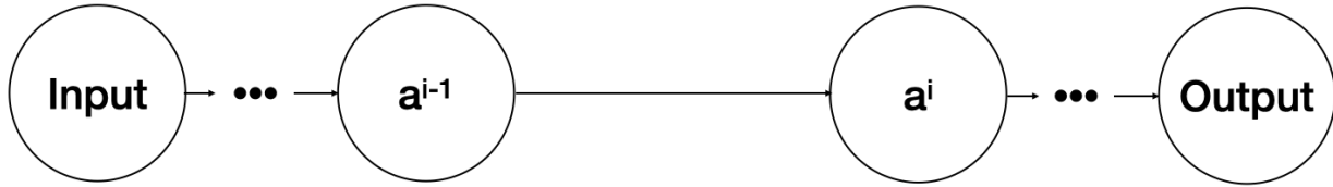
Figure 2.5: Sketch of a neural network with any number of layers, each featuring one single neuron. Depicted are the Input and Output, along with two neighbouring layers, called i and i-1 . Since there is only one neuron per layer, each activation can be found iteratively by equation 2.2
