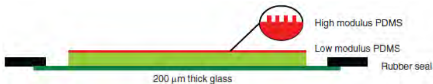
Figure 3.1: SCIL stamp based on PDMS silicone rubber applied on glass. With SCIL, rigid glass and soft PDMS-rubber together combine advantages of rigid and soft stamps used for nano-lithography. Graph by [VMN + 17]
