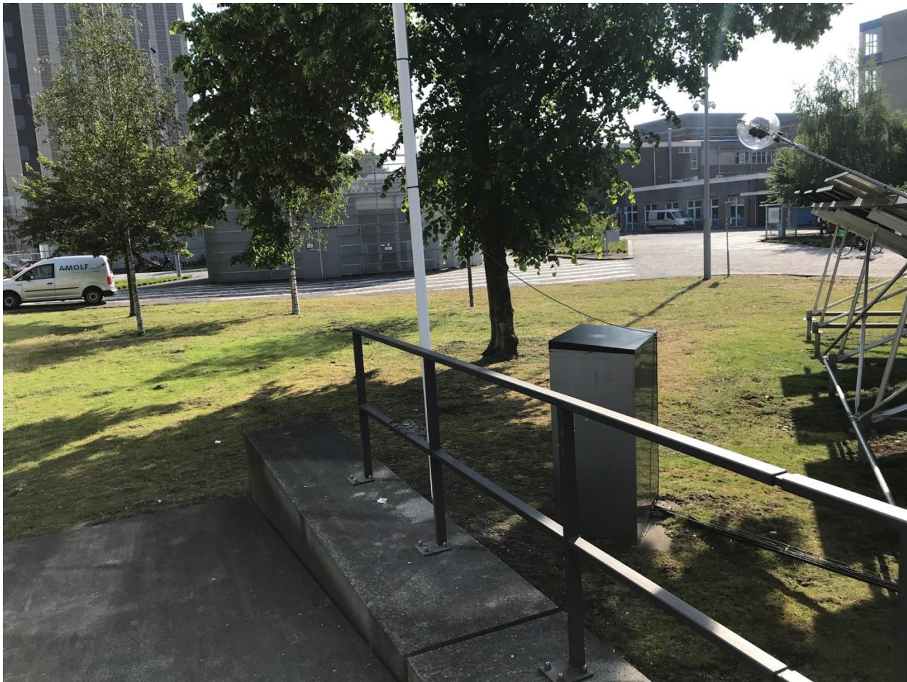
Figure 3.1: The image shows the surface background behind the AMOLF solar field. The presence of concrete, grass and shade from the near tree complicates the calculation of the albedo value, which influences the reflected light detected by the rear side of the LAD. A rough estimate constrains the albedo value between 0.1 and 0.2.
